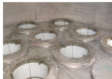
Mist Eliminator Raised Flange Design
