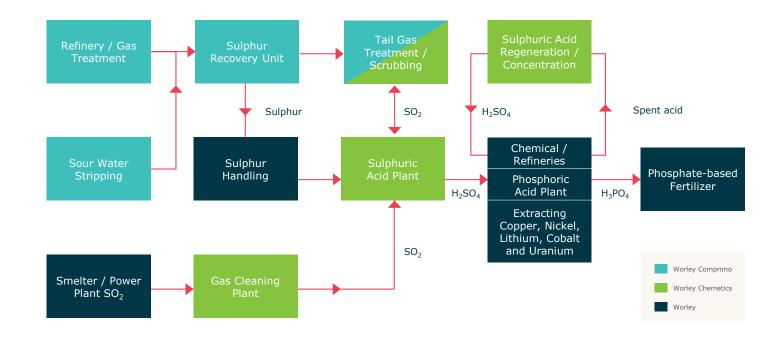
Together, we deliver technologies for all forms of sulphur species, from H<sub>2</sub>S to sulphur, sulphur via  $SO_2$  to sulphuric acid and sulphur handling and transportation.
